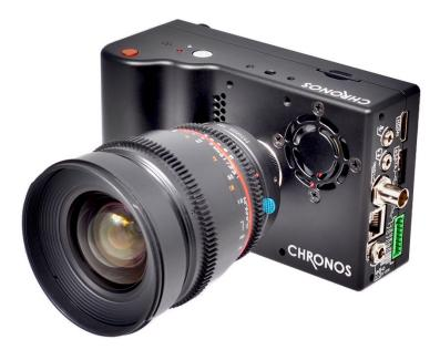
Chronos 2.1-HD is a 1080p, 2.1 gigapixel-per- second handheld high-speed camera. Completely self-contained, you can take high-speed imaging with you anywhere! It records 1080p video at 1000fps, and can record at up to 24 046fps at lower resolutions. Video is saved to removable media in compressed h.264 or uncompressed dng format. You can shoot for hours, saving hundreds of shots on a single card.
